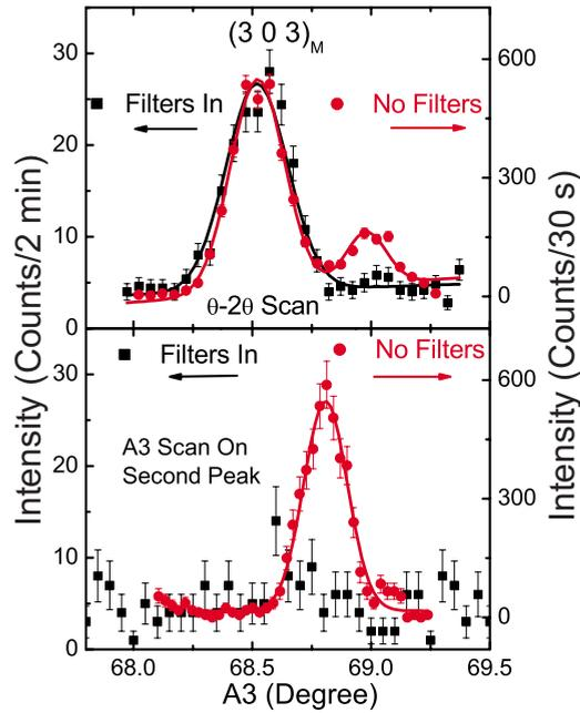
FIG. 3. (Color online) (a) Rocking curves of the (3,0,3) magnetic Bragg peak, and its comparison with structural Bragg peaks obtained from  $\lambda/2$  of the nuclear (6,0,6) and (0,6,6) reflections. (b) Identical rocking curve for (0,3,3) magnetic peak position showing no magnetic scattering. This provides definitive evidence that the AFM order occurs along the  $a$ -axis direction.
